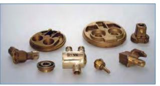
This involves shaping a billet of brass, heated in advance to a temperature of 600–750 °C depending on the type of brass. This operation is carried out on a press fitted with a machined tool corresponding to the general shape of the part to be obtained. The rough produced can be machined to obtain the finished part required.
